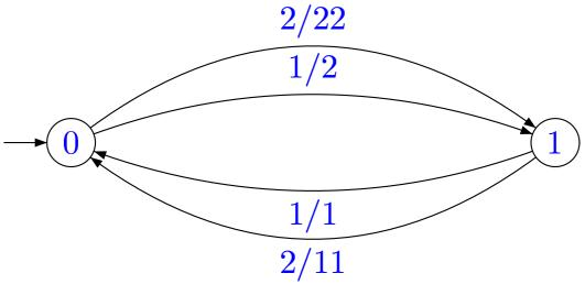
The sequential machine can be viewed as a special case of a Tag machine, when reading and writing on the same tape.
