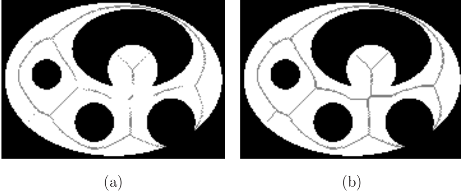
Fig. 13. (a): a subset S of \mathbb{G}^2 (in white) and its medial axis \text{MA}(S) (in gray). (b): in gray, AK^2(S) .
