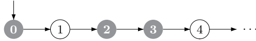
Fig. 12: Automaton for the Fibonacci infinite word f . A state i is final if f_i = a . The state 0 is initial. Final states are gray.
