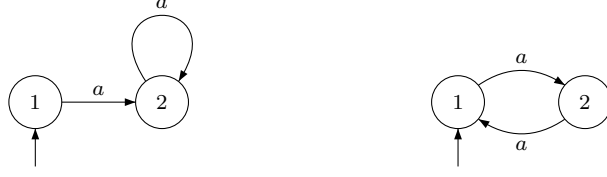
Figure 5: On the left, the sets of final states \emptyset and \{1\} are not possible for the automaton to be co-accessible. On the right, only the empty set is not allowed.
