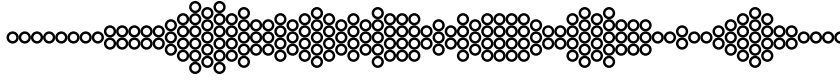
Fig. 3. The shape of a random acyclic automata with 200 states on a two-letter alphabet. The initial state is on the left, and we have represented the number of sources seen at each step when repeatedly pruning the automaton. The width of this automaton is 6, and its shape is typical of what is observed under the uniform distribution.
