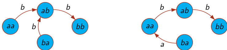
Figure: The two spanning trees of de Bruijn graph of order n = 3 with root bb .
