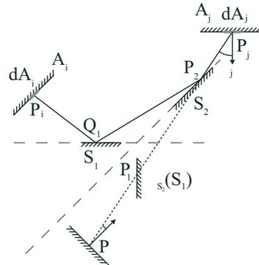
Figure 5: Calculation of a form factor of level 2.
