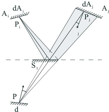
Figure 4: Calculation of the extended form factor
