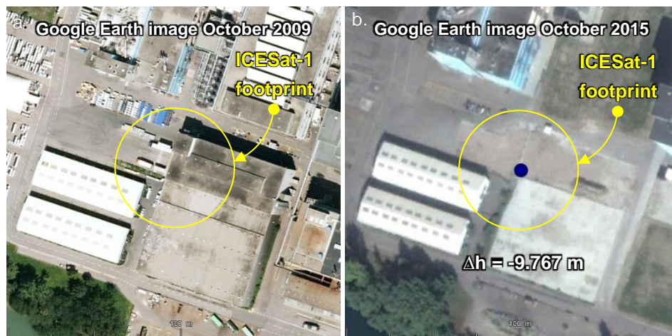
Figure 27 - EEA-10 - ICESat-1 height differences – Demolition of an industrial building over two acquisition dates.
