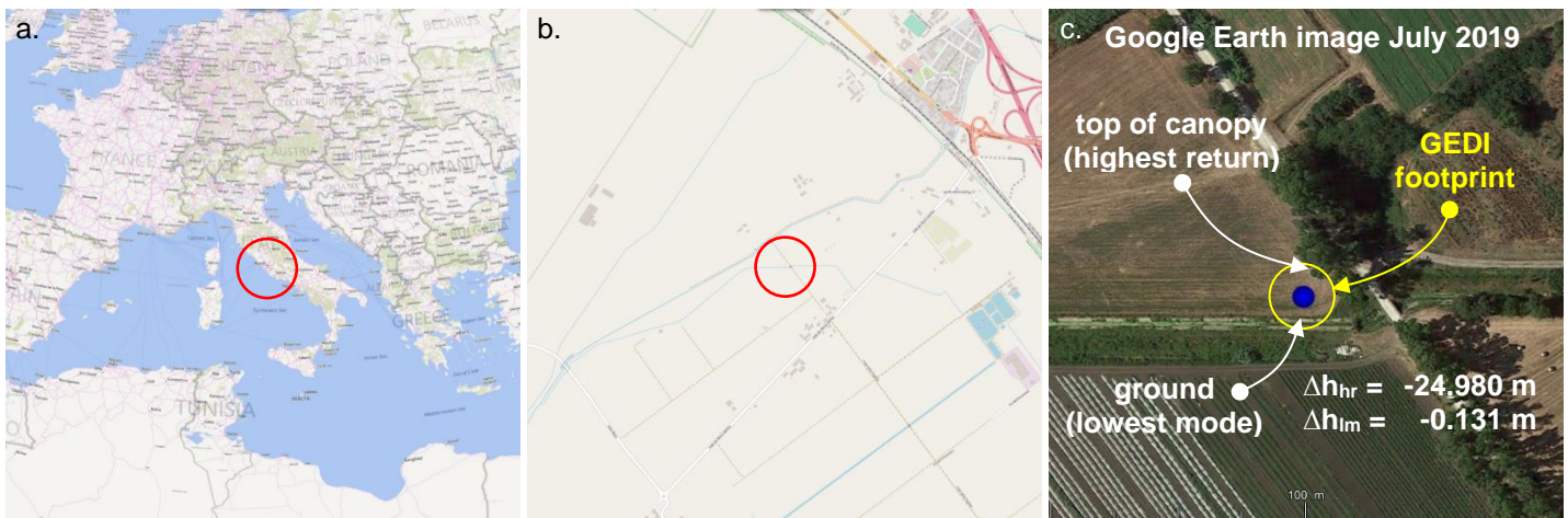
Figure 67 - EEA-10 - GEDI height differences – Case of sparse canopy near fields of Centro Tre Denari (Italy).
