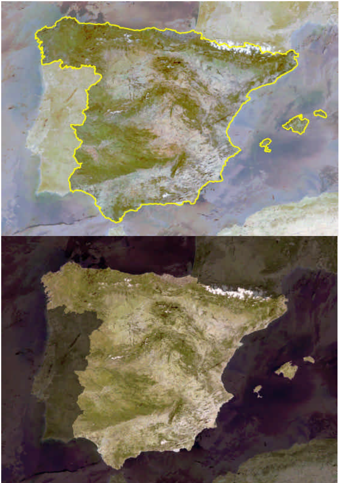
fig. 87 - Spain – Projection UTM 30 Up: bands 3-5-7 – Bottom: bands 3-5-pca1 (first principal component analysis).
