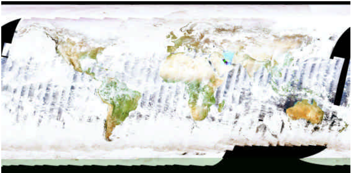
fig. 25 - “Replacement” merging algorithm - “NDVI maximum” selection algorithm.
