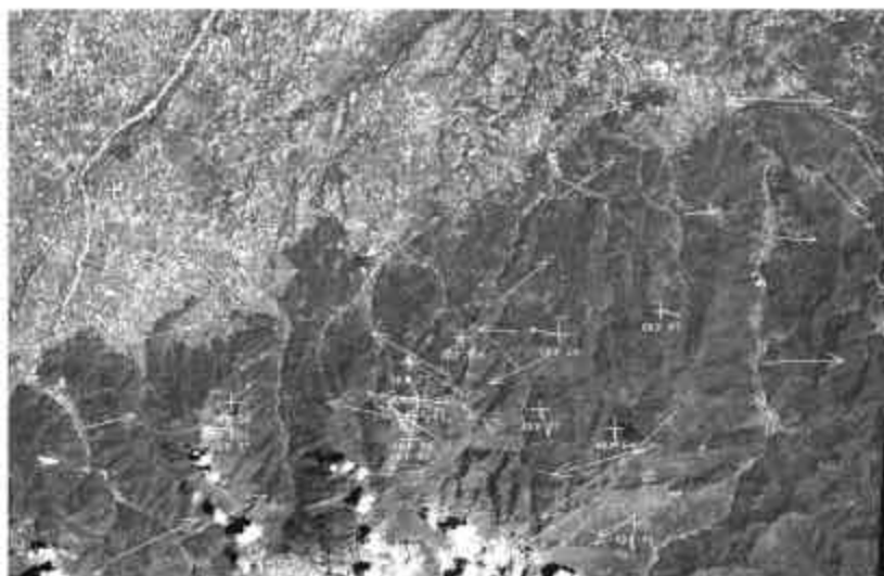
Figure X.11. Defects of parallax corrections in a mountainous area.
