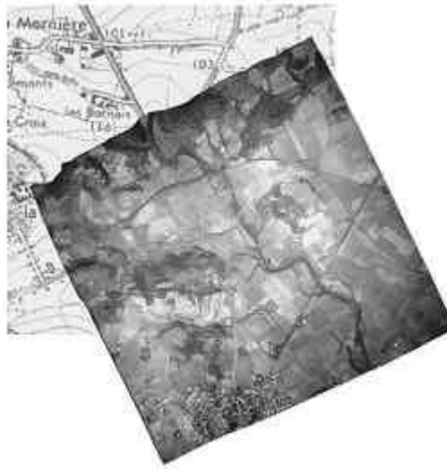
Figure X.1. Orthorectified aerial photograph superposed on a map. (Courtesy TTI Productions).
