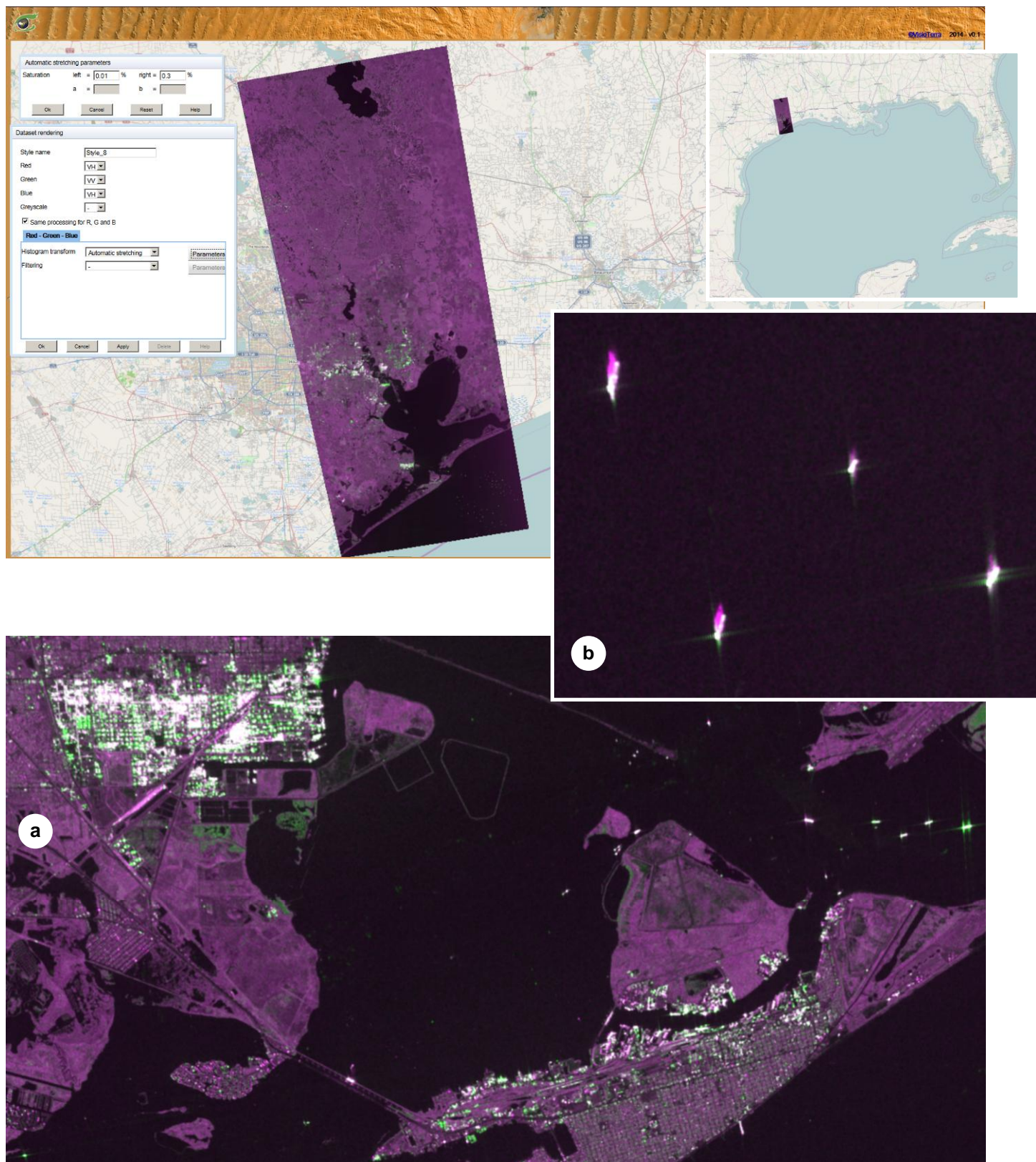
fig. 46 - Display in ViWeb of a SM product over Houston (Texas) - Simple 0.01-0.3 automatic stretching highlighting buildings with metallic structures like the Texas City oil refinery (a) and ships waiting at the entry of Galveston Bay (b).
